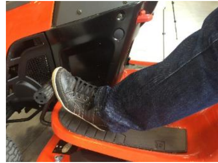
Pressing the brake pedal must automatically disengage the freewheel
