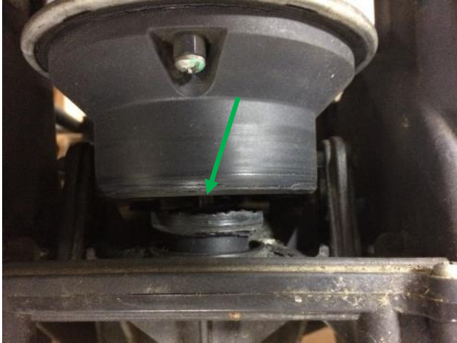
Damaged primary pulley
