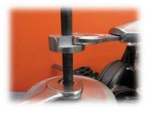
Make sure not to lose the 8 balls under the flange
