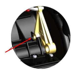
8- Make sure that the variator pulley rotates freely, then install the drive belt in the pulley
