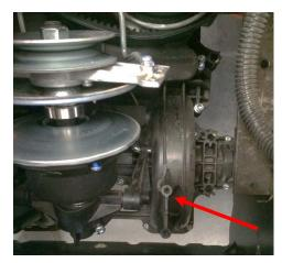
5- Install the variator lever on both sides of the variator pulley.
