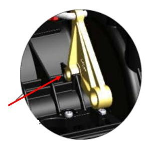
7- Make sure that the variator pulley rotates freely, then install the drive belt in the pulley
