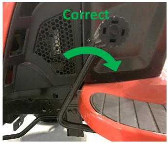
III- Check for debris impeding movement of the brake pedal to full back position.
