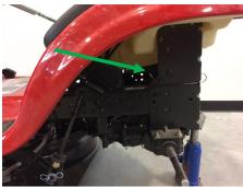
Remove the belt from the transmission pulley
