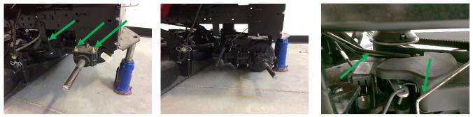
Carefully, slowly removed the transmission as the pedal rod and freewheel rod are still connected.
