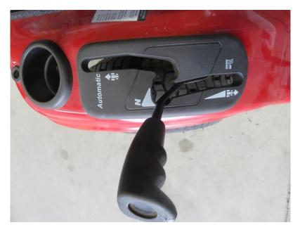
A successful adjustment will allow moving the tractor by hand by using the bypass and Neutral lever with no more than the normal "purring" gear sound from the transmission.
