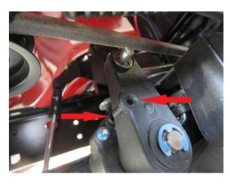
2. The "neutral" position of the fender control lever can now be checked. If the lever has been moved somewhat to the "Forward" or "Reverse" direction to allow the tractor to be rolled by hand, the linkage requires adjustment. A proper "Neutral" position is shown below.
