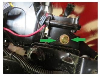
With the 4MM pin or Allen wrench in place, Loosen and adjust this bolt and bracket in the slot so the lever is in the "Neutral" position, then tighten it.
