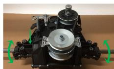
If the transmission cannot perform these 3 steps, the transmission needs to be replaced
