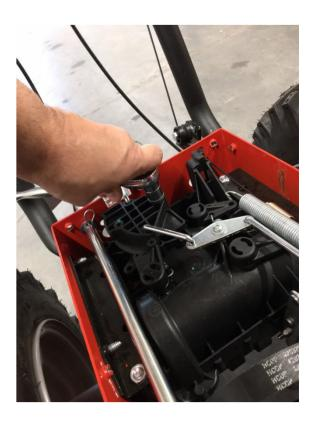
\*Tighten bolt to 3.7 ft.·lbf/5.0Nm
