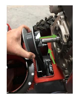
Put pulley back on driveshaft
