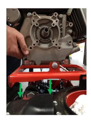
Place engine on unit, install belt on drive pulley
