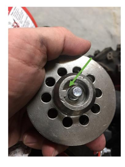
Be sure to match notch on pulley to notch in driveshaft
