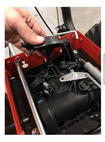
Place new cam on shaft and rod into lever
