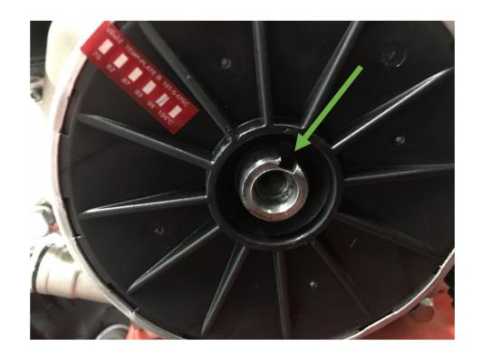
\*Torque engine pulley bolt to 23-29 ft-lbs/31-39Nm
