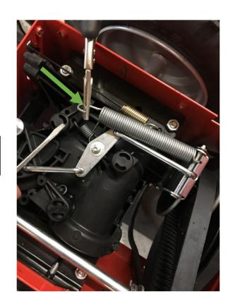
Remove cam bolt w/ 13mm wrench
