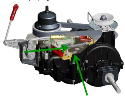
**P8** -To remove the transmission, disconnect the variation rod (1) from the friction pack.
