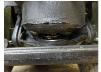
Secondary pulley axle worn
