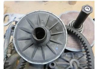
Damage caused by incorrect drive belt routing
